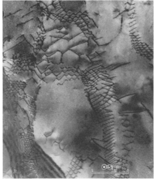
Figure 9 16% deformed and annealed 1 h at 1050° C. Note polygonised cell structure.
