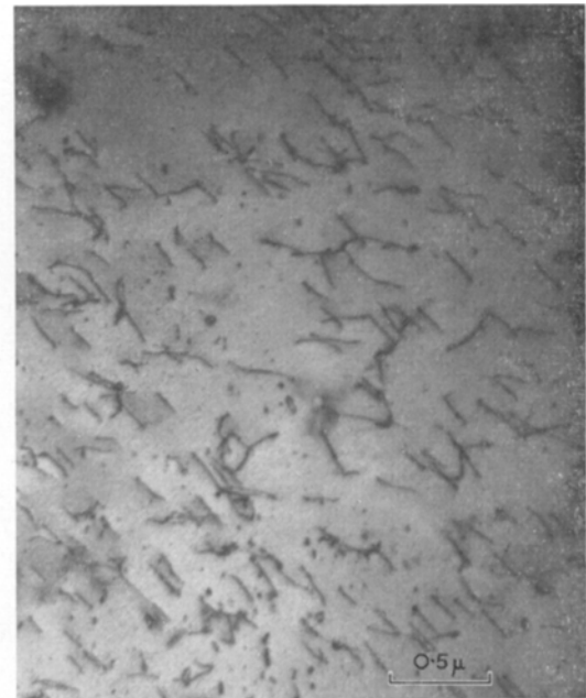
Figure 5 Electron micrograph after 4% deformation.
