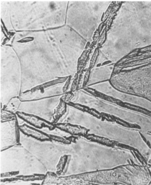
Figure 3 Optical micrograph of Mo/Re alloy after 27% deformation showing notched twins.
