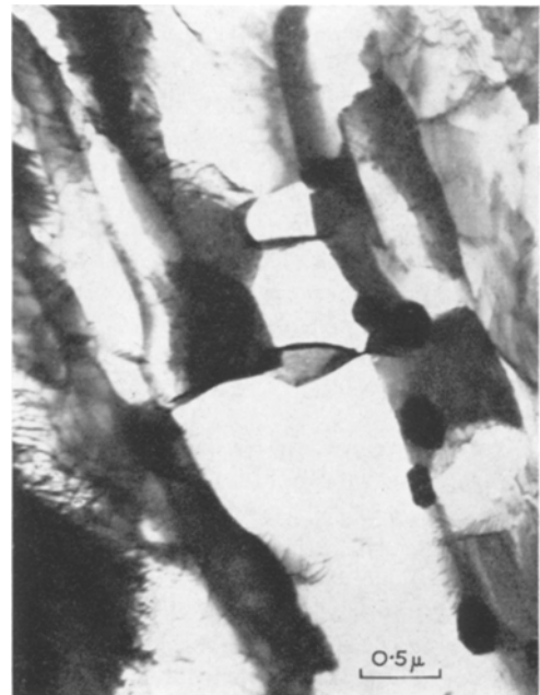
Figure 10 16% deformed and annealed 1 h at 1200° C, showing precipitates of sigma-phase.
